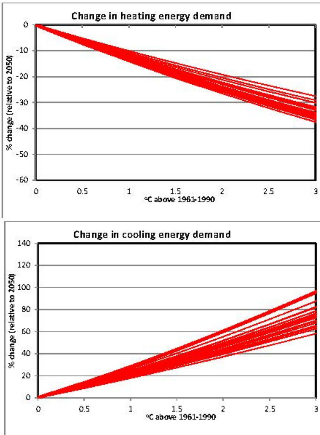
Figure 2.7. Damage function showing change in residential heating and cooling demand in 2050 with global mean temperature change (relative to 1961-1990). The different lines represent different climate model patterns. Arnell et al. (2014).
