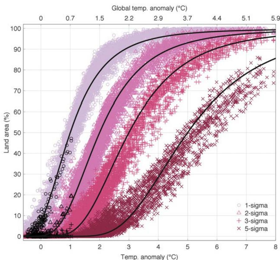
Figure 2.3.2. Damage function showing the proportion of land area with summer temperatures more than one, two, three or four sigmas from the 1961-1990 mean (Coumou & Robinson, 2013). The individual symbols represent individual model years. Global mean temperature change (relative to 1951-1980) is shown along the top horizontal axis; the bottom axis shows land temperature change.
