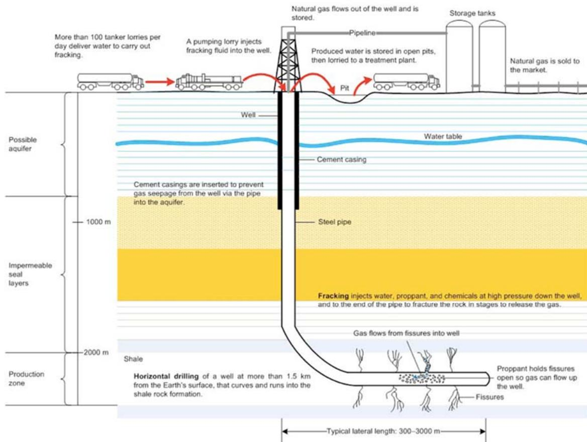
**Figure 1: Shale gas operation with fracking, reproduced from Hirst et al. [5], adapted from Granberg [6].**
